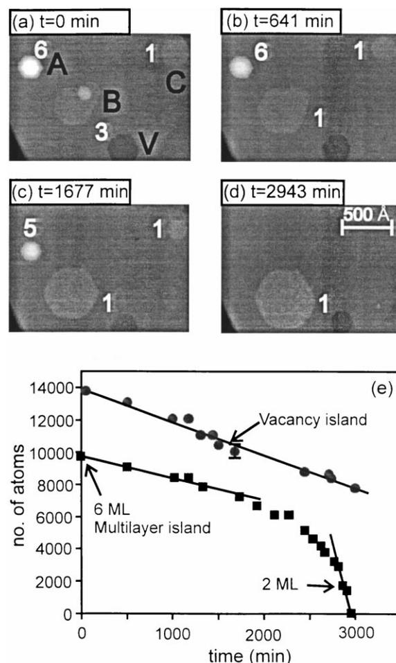
Fig. 3. (a)–(d) Representative images showing the decay of multilayer island A, the growth and shape change of B, and the partial filling of the vacancy island. Sample bias  $1.0 \text{ V}$ , tunneling current  $0.5 \text{ nA}$ . (e) The number of atoms in base layer of island A during its decay and the rate of filling of the vacancy island.
