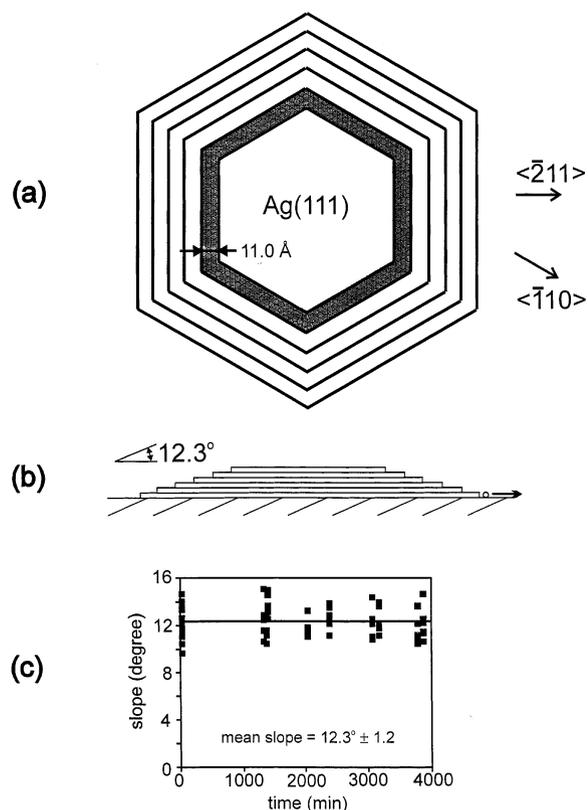
Fig. 2. (a) Top and (b) side view of a multilayer island of Ag that had wet the Ag(111) surface. The average slope was  $12.3 \pm 1.2^\circ$  and this was maintained during island decay (c). The mean terrace width was  $11 \pm 1 \text{ \AA}$  ( $3.8 \pm 0.3$  atom diameters).
